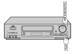
Your VCR is equipped with the TimeScan function. TimeScan allows noise free pictures to be displayed on your TV screen in the forward and reverse search modes. Audio will be played back at normal speed during any of the TimeScan modes (F) pg. 35). TimeScan allows you to view a program in search mode while listening to the audio.
